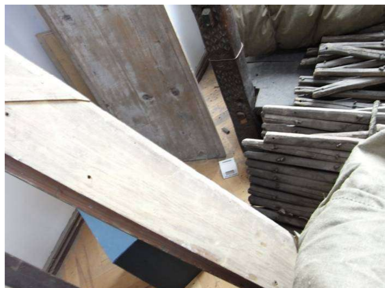
Fig 8-9: Infested wood objects from a wood boring beetle (probably Anobium sp ) in the Janashia building.
